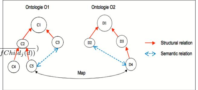
Figure 5: Example of ontologies with semantic relations allowing to generate new mapping candidates. Because we have a validated mapping  $Map$  between  $C5$  and  $D4$ , a candidate mapping could be generated between  $C3$  and  $D2$  by the semantic matcher since there is a same semantic relation between  $C5$  and  $C3$  and between  $D4$  and  $D2$  (this relation could be a relation generated by the enrichment phase).
