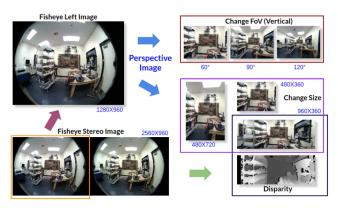
established. Existing algorithms for conventional stereo vision can thus be adapted for fisheye stereo images. The proposed technique will be evaluated using the stereo fisheye camera from ATAR. A comparison with traditional stereo cameras will be realized.
