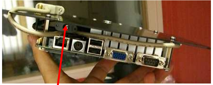
Connector to plug-in the embedded CPU
