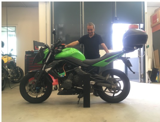
FIGURE 3.5: The instrumented Kawasaki ER6N PTWV.
