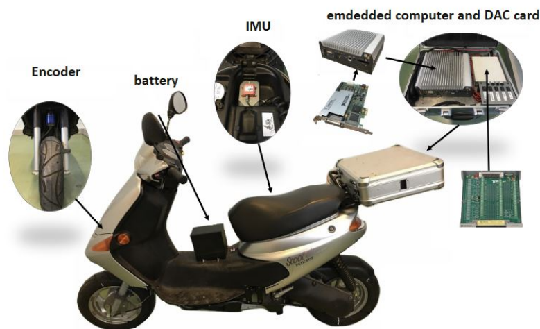
FIGURE 2.21: Instrumented Scooter at the IBISC Lab, university of Evry.
